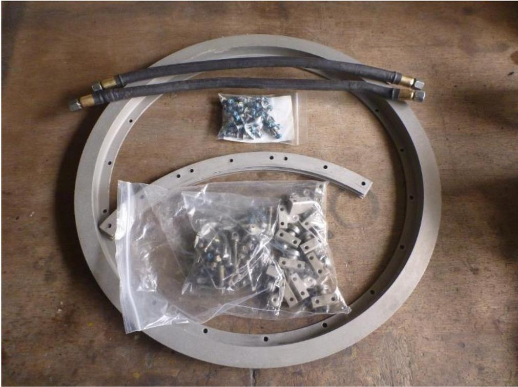
Seen below are the cleaned and packed components from the main turret rings. In bags there are the special bolts, vertical rollers and horizontal rollers. Above them the turret rotation stops and turret lock castings. Again, these were in very good condition especially given the corrosion found on the actual turret rings.
