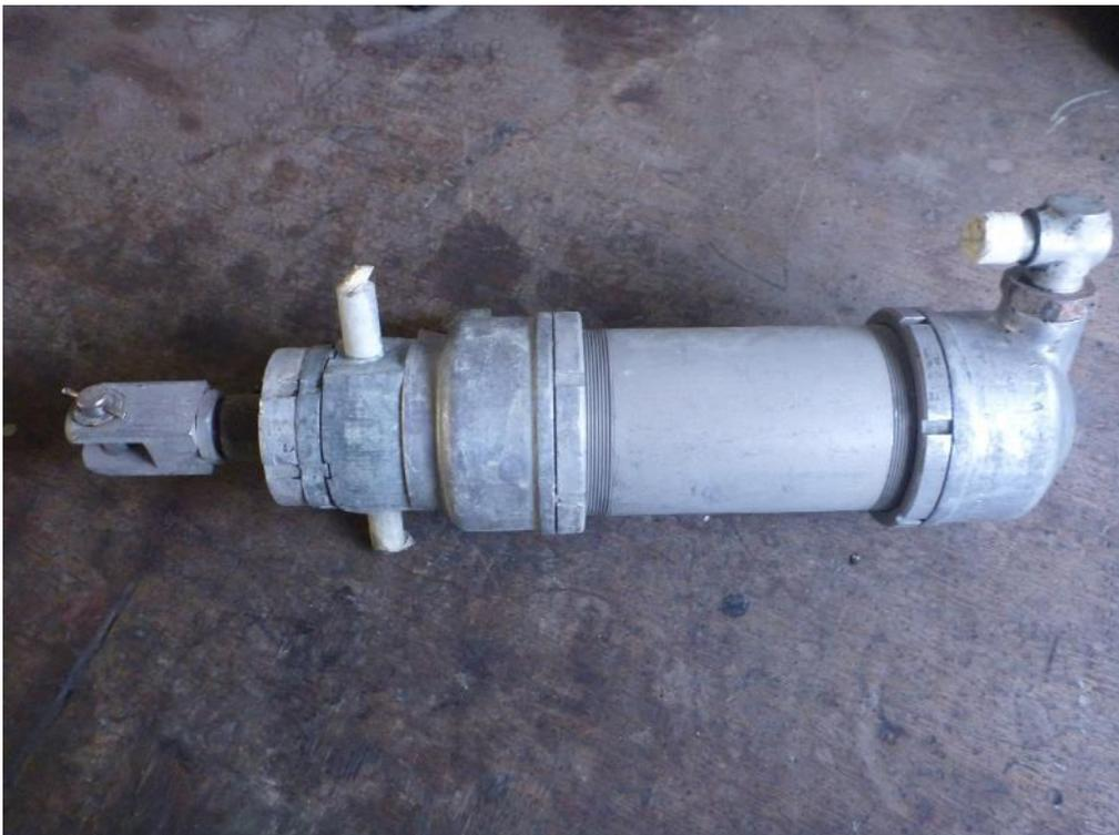
The view above is of the main (elevation) ram which also benefitted from a good clean before being prepared for painting.
