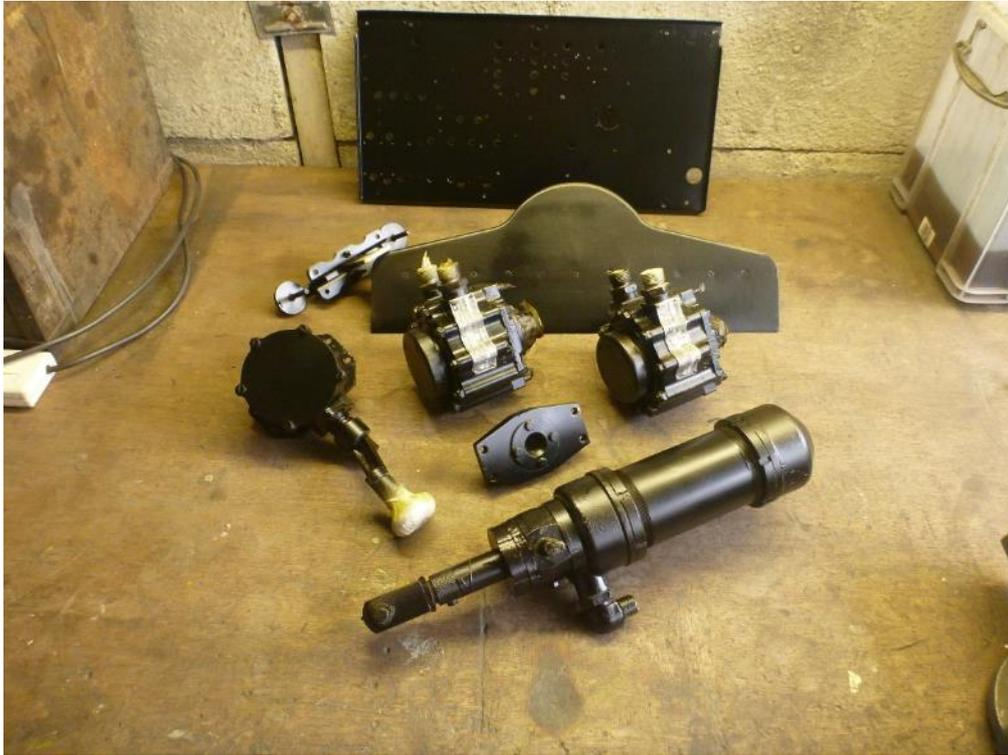
Next on the agenda were the components removed from the damaged drum and floor assembly. Within the floor assembly there is a fixed floor that does not rotate with the turret and so has a number of horizontal and vertical rollers to allow this to happen.
